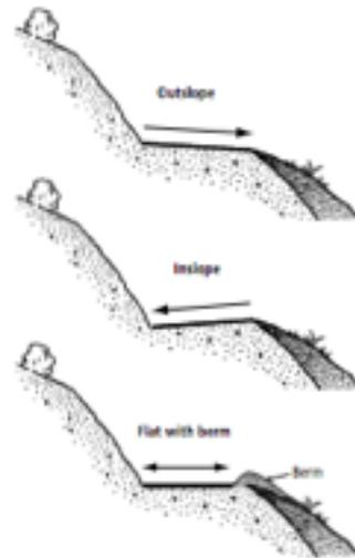
Figure 13-9. Outslope, inslope, and berm.
