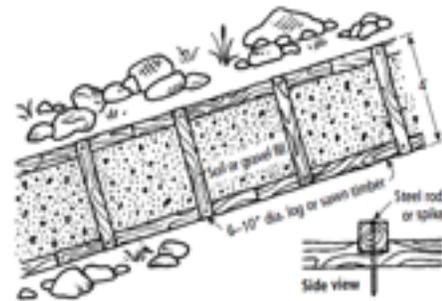
Figure 13-13. A climbing causeway allows you to hold fill material on a steep grade.
