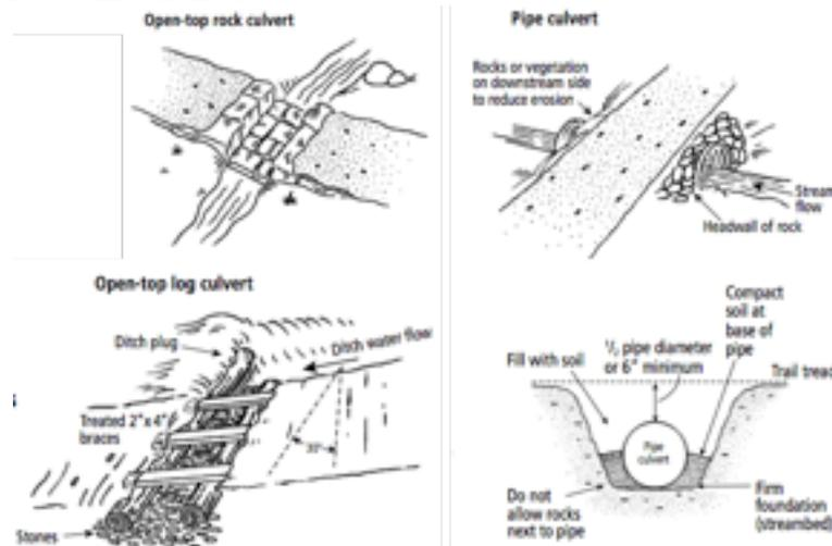
Figure 13-22. A culvert is a good option for crossing a narrow stream.
