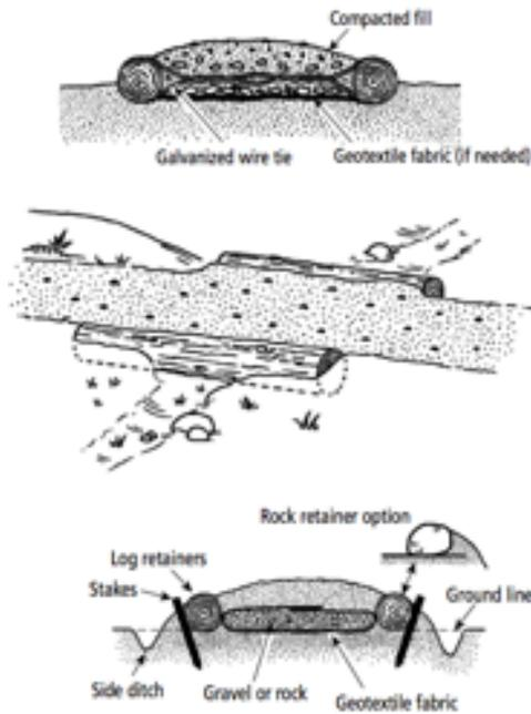
Figure 13-18. A causeway (turnpike) raises the tread above wet soil.
