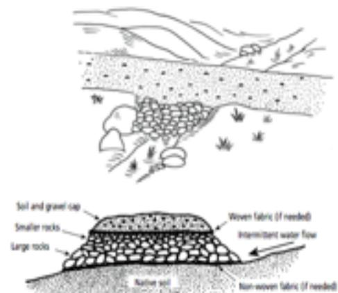
**Figure 13-17. A drainage lens allows water to seep beneath the tread.**
