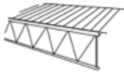
Figure 13-24. Girders and trusses support the bridge deck.
