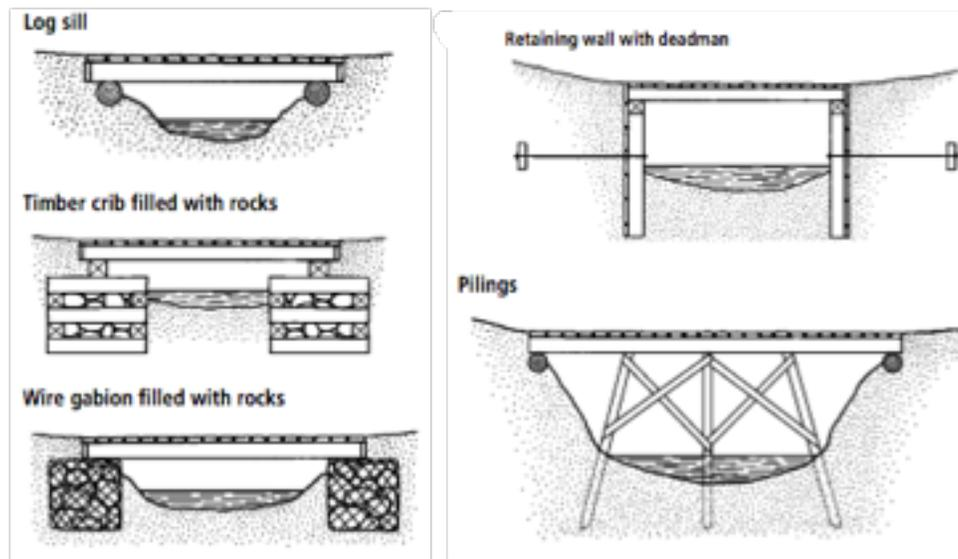
Figure 13-23. The best type of abutments for your bridge depends on the size of the bridge and the surrounding conditions.
