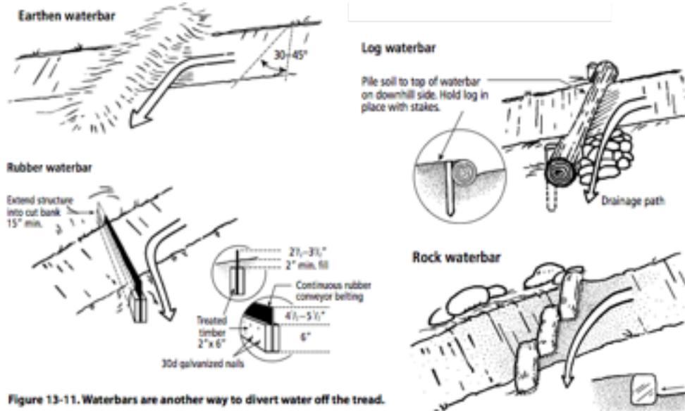
Figure 13-11. Waterbars are another way to divert water off the tread.
