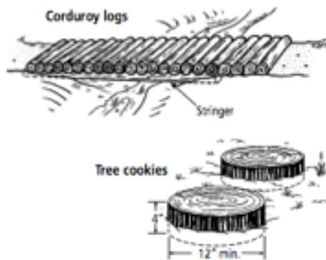
**Figure 13-16. Corduroy logs and tree cookies are inexpensive ways to raise a tread in wet soil but they are slippery to cross.**
