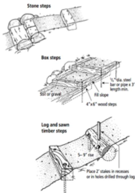
Figure 13-14. Steps help prevent erosion and make it easier to navigate a slope.
