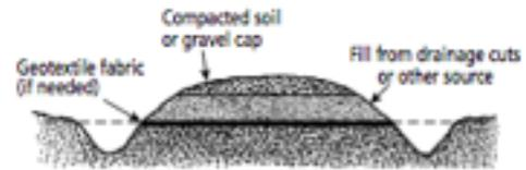
Figure 13-19. Center crown with ditches.
